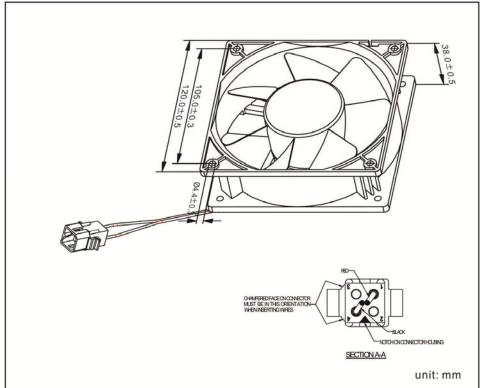
With Molex Connector: Housing# 46999-0652 Terminal# 0039000283
