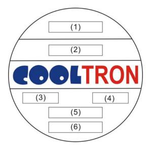
(2)Model Number & Appendix Code(3)Rated Voltage(4)Power Consumption(5)Bearing Type(6)Location
